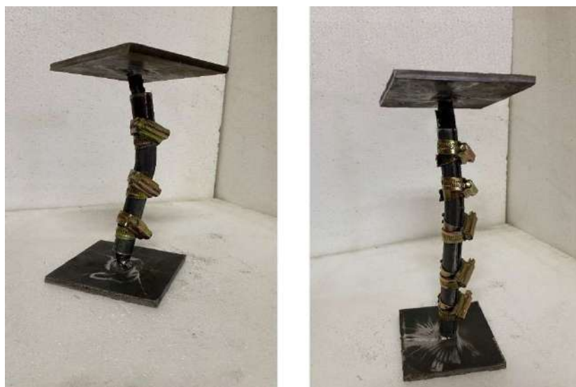
Figure 3. 35 Specimen (W – 15 - 6 Φ), (W – 25 - 6 Φ) Fail Shape
