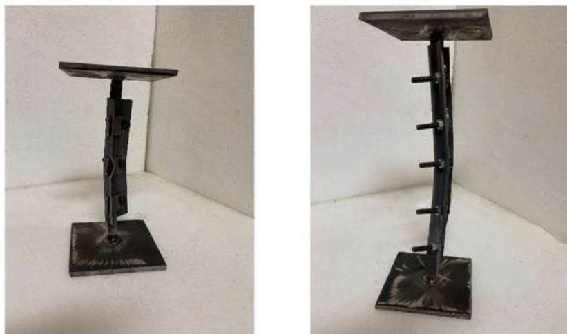
Figure 3. 31 Specimen (S – 15 - 6 Φ), (S – 25 - 6 Φ) Fail Shape
