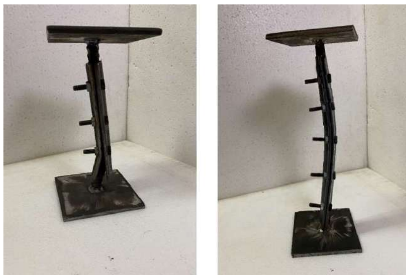
Figure 3. 27 Specimen (F – 15 - 6 Φ), (F – 25 - 6 Φ) Fail Shape
