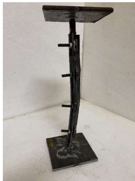
Figure 3. 48 Specimen (S – 25 - 9 \Phi ) Fail Shape
