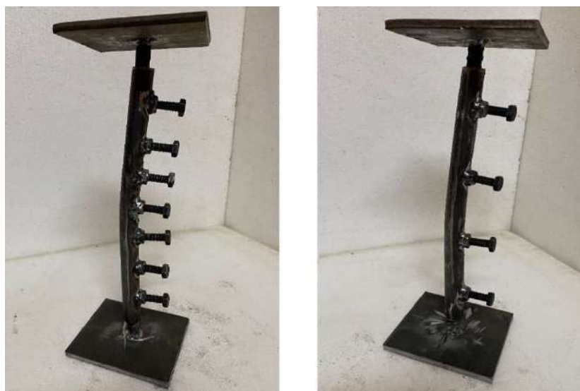
Figure 3. 56 Specimen (N – 25 - 3 \Phi ), (N – 25 - 9 \Phi ) Fail Shape
