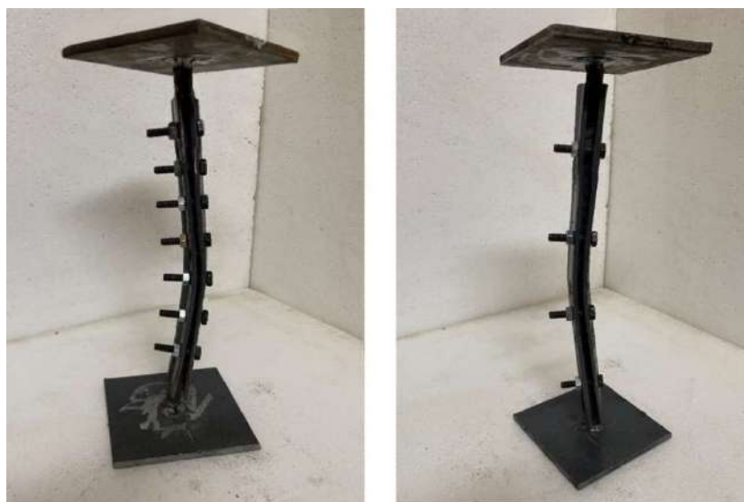
Figure 3. 44 Specimen (F – 25 - 3 Φ), (F – 25 - 9 Φ) Fail Shape
