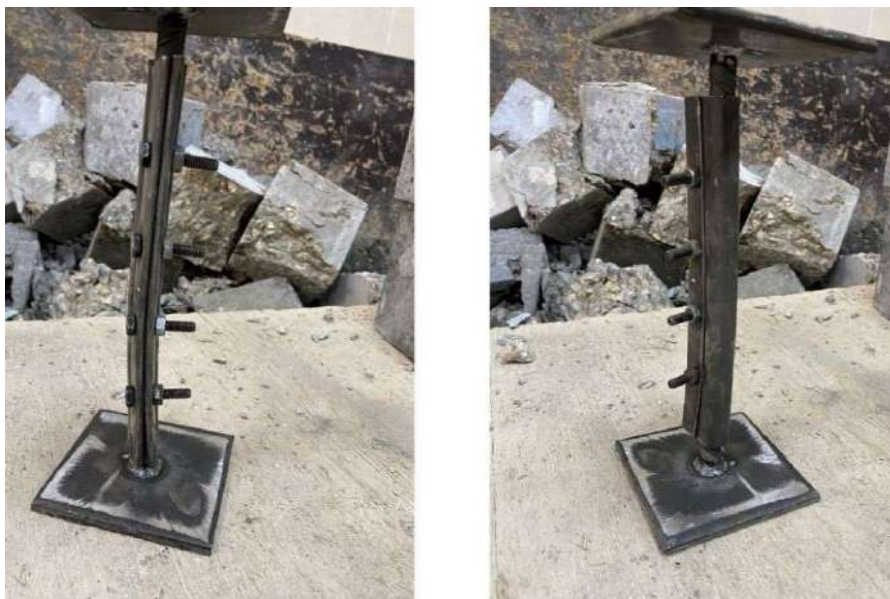
Figure 3.14 Specimen (F – 20 - 6 Φ) Failure Shape
