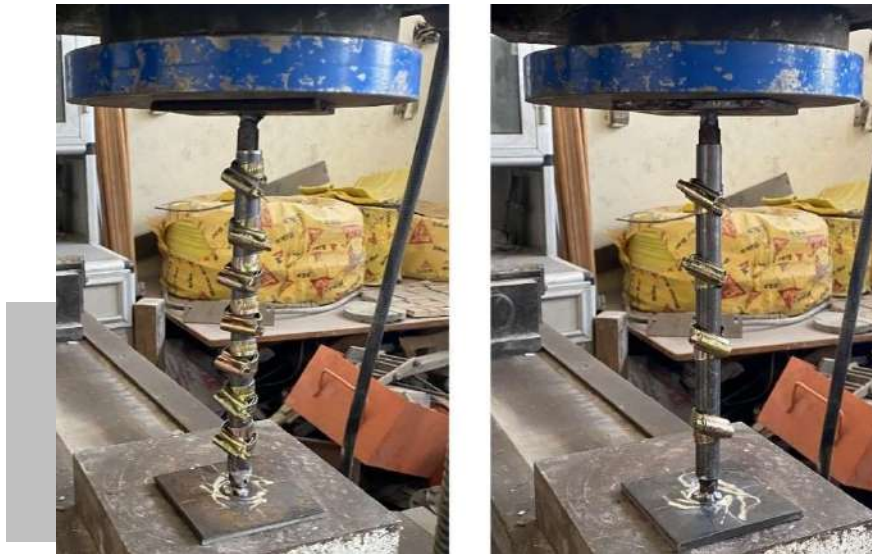
Figure 3. 51 Specimen (W – 25 - 3 Φ), (W – 25 - 9 Φ) Testing
