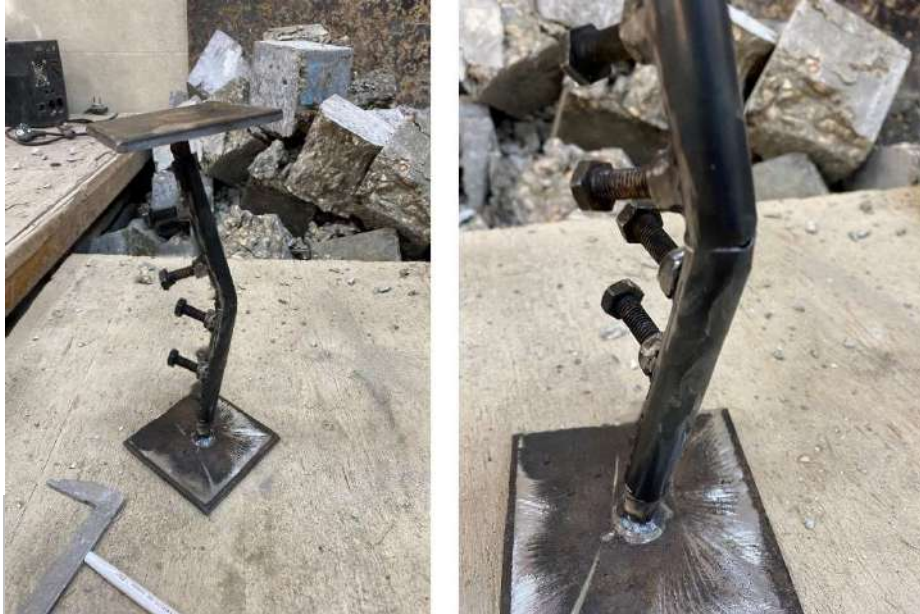
Figure 3. 23 Specimen (N – 20 - 6 \Phi ) Failure Shape
