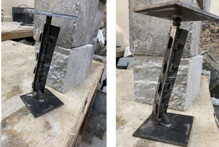
Figure 3. 17 Specimen (S – 20 - 6 \Phi ) Failure Shape
