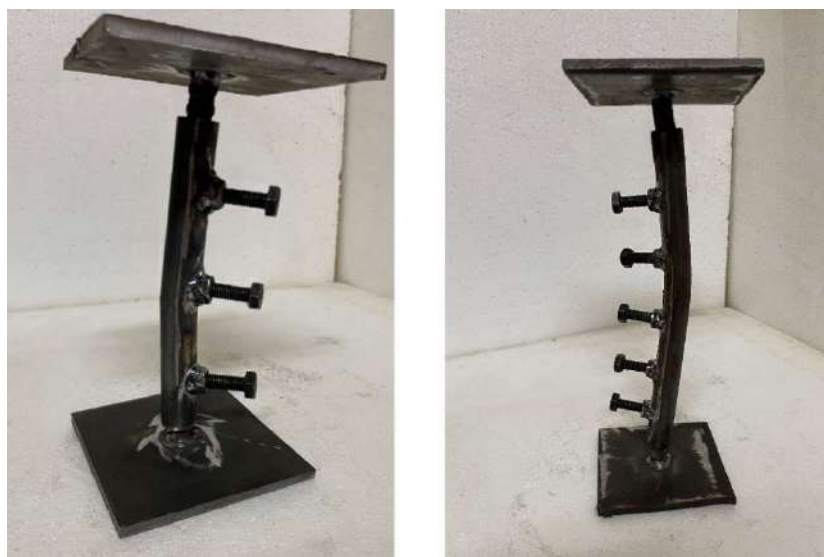
Figure 3. 39 Specimen (N – 15 - 6 Φ), (N – 25 - 6 Φ) Fail Shape
