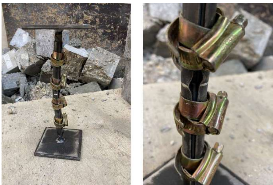
Figure 3. 20 Specimen (W – 20 - 6 Φ) Failure Shape
